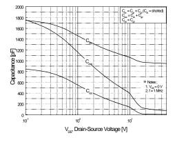
Figure 5. Capacitance Characteristics
