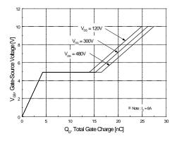
Figure 6. Gate Charge Characteristics
