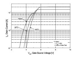
Figure 2. Transfer Characteristics
